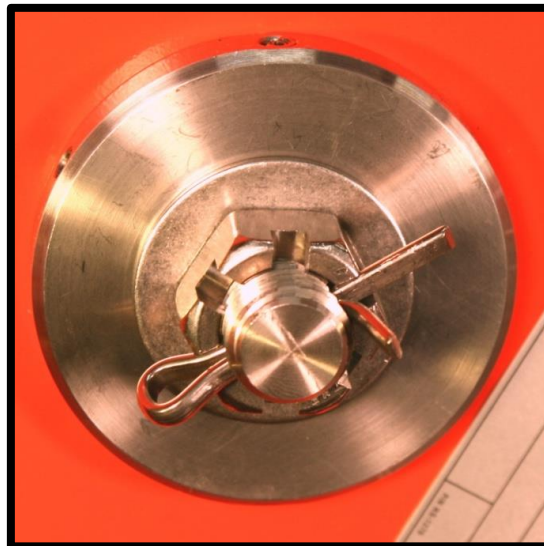
Properly Locked Pivot Pin Figure 27
