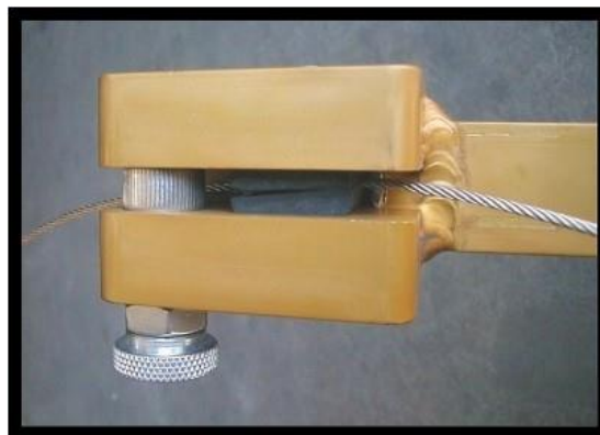
Figure 22 Loading the Slickline Figure 23 Installing into Wiper
