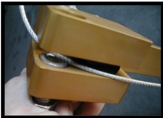
Figure 22 Loading the Slickline Figure 23 Installing into Wiper
